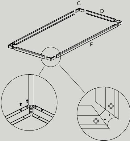
**NB!** Make sure the holes on the corner (C) are facing up.
